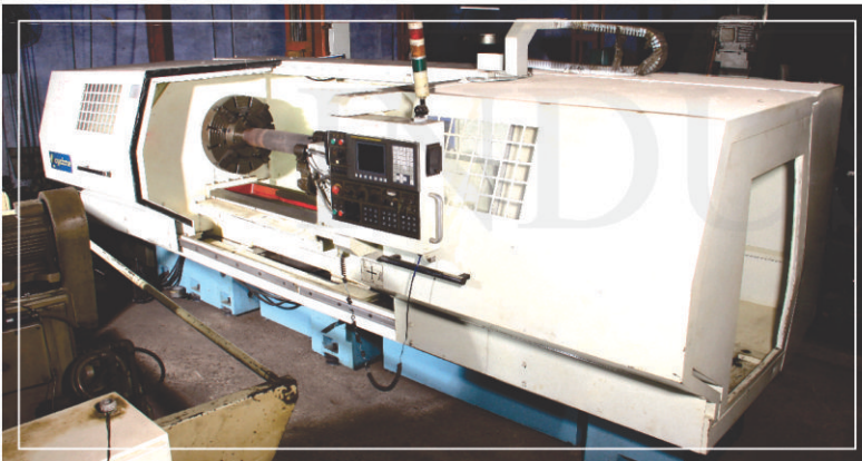
CNC M/c 10mm Dia to 600mm Dia length up to 5 mtr.
